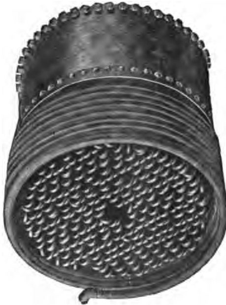
FIG. 171. —Improved Rider Boiler. The same J-tubes are used in this generator as are shown in a former figure, except that, instead of being inserted into plugs, as there shown, they are expanded evenly into the crown sheet; thus giving a much larger heating surface. The feed water circulates through the coil surrounding the tube area, thus insuring its pre-heating. Rapid steaming qualities and very high efficiency are claimed for this type of generator, which can develop 6\frac{1}{4} horse-power on 16'' \times 16' dimensions, over all, and 5 horse-power on 14'' \times 14'' dimensions.
